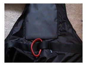
The main purpose of this connection is as a temporary tether to the tower or as a redundant connection to the zipline cable. This loop must **NEVER** be used as the main zipline hook in point. The harness will continue to work, if this loop is used as the primary point, however the stitching will start to tear and the harness will need to be repaired or replaced.
