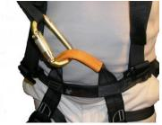
The hook in points will eventually wear out and the harness will need to be replaced, once the protective orange cover is worn through, and you can see the black webbing – the harness MUST be retired. The complete harness should be inspected daily for any problems (rips, cuts or abrasion).
